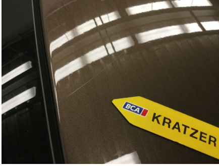
EXTERIOR - ROOF Roof; Scratched; Over 25mm Thru Paint
